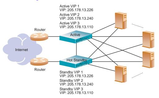
Figure 11-6 Hot-Standby Redundancy
